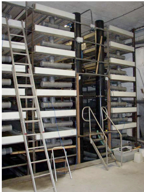
Figure 2: Seven-level shallow tanks for sole ( Solea solea ) production at Solea BV in The Netherlands (Photo credit: Albert Imsland, Akvaplan-niva)
