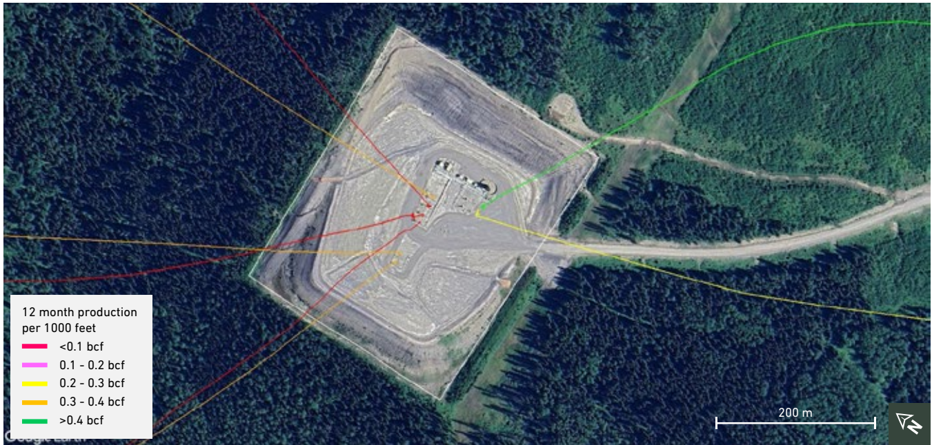
Figure 23 – Closeup of a well pad containing eight horizontal wells on 8.54 ha, which is fairly typical of the North Montney subarea. The location of this well pad within the North Montney subarea is indicated in figures 21 (lower star) and 22 (white outline). The productivity of individual wells is indicated by well trajectory colour.
